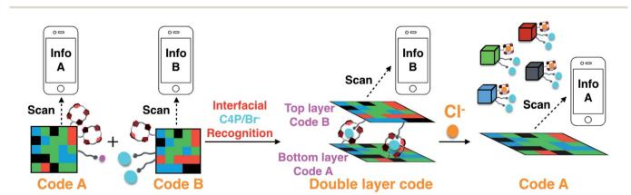
Scheme 1 Formation of a double layer code construct stabilized *via* presumed interfacial anion-receptor interactions involving the recognition elements present in Code A and Code B. Also shown is the proposed Cl<sup>-</sup> anion induced delamination and encoded information release-based sensing mechanism that allows for chloride specific anion sensing.
