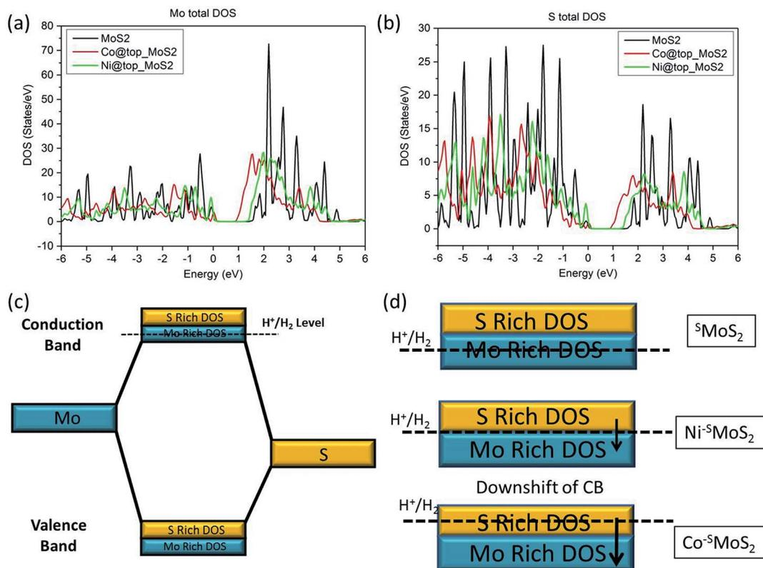
Fig. 7 Calculated Density of States (DoS) of (a) Mo and (b) S in <sup>S</sup>MoS<sub>2</sub>, Co-<sup>S</sup>MoS<sub>2</sub> and Ni-<sup>S</sup>MoS<sub>2</sub> (c) simplified molecular orbital diagram of MoS<sub>2</sub> (d) downshift of the conduction band (CB) upon addition of a single Co and Ni metal atom at the Mo atop site, respectively.
