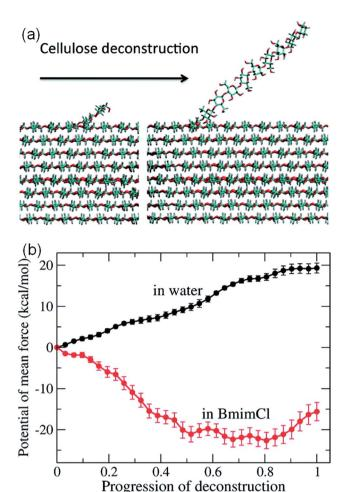
Fig. 16 (a) The peeling process of cellulose by means of steered molecular simulation. (b) The potential mean force (PMF) of the peeling process in water and ionic liquids. 99 Reproduced from ref. 99 with permission from the American Chemical Society.
