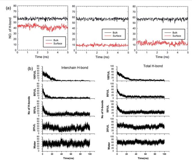
Fig. 12 (a) The change of H-bonds inside the cellulose layer (black) and at the surface (red). From left to right is [Bmim][PF<sub>6</sub>], [Bmim][OAc] and  $H_2O.^{94}$  (b) Effect of [C<sub>2</sub>mim][OAc]—water mixtures on the disruption of the inter-chain H-bonds and total H-bonds between cellulose at 160 °C.<sup>42</sup> Reproduced from ref. 42 and 94 with permission from Elsevier and the Royal Society of Chemistry.
