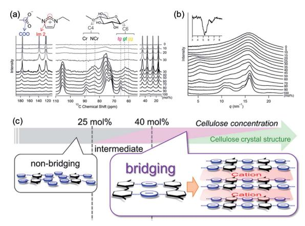
Fig. 5 (a) <sup>13</sup>C solid-state NMR spectra obtained at 5 kHz of MAS for the cellulose/[Emim][OAc] mixtures. (b) WAXS patterns of cellulose/[Emim] [OAc] mixtures. (c) Schematic summary of non-bridging to bridging state transformation with the increase of cellulose concentration in [Emim] [OAc]. For Reproduced from ref. 50 with permission from the American Chemical Society.
