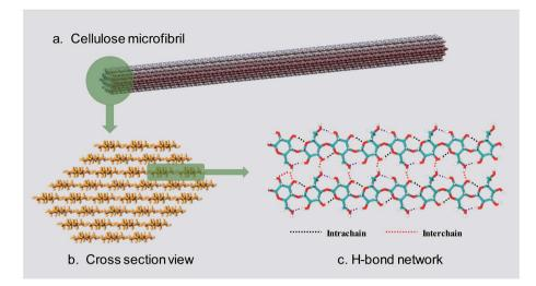
Fig. 1 (a) The usual form of existence of cellulose—cellulose microfibril. (b) Cross-section view of a 36 chain cellulose elementary microfibril. (c) The H-bond network between cellulose chains.
