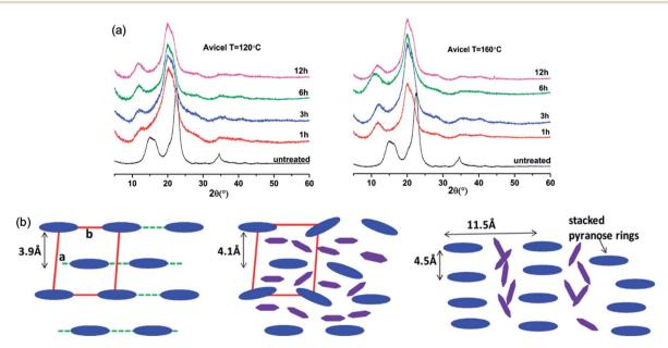
Fig. 6 (a) XRD patterns of Avicel cellulose in [Emim][OAc] at  $120 \,^{\circ}$ C (left) and  $160 \,^{\circ}$ C (right).<sup>55</sup> (b) Schematic representation of the arrangement of cellulose crystalline structure (blue) and the intercalated ILs (purple).<sup>56</sup> Reproduced from ref. 55 and 56 with permission from the American Chemical Society.
