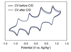
Fig. 6 CV of complex 6-V<sub>6</sub>O<sub>7</sub>(OEt)<sub>12</sub> before and after cycling.
