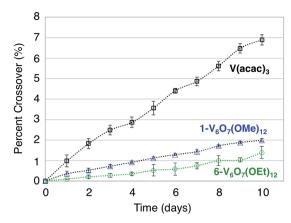
Fig. 7 Extent of cross over for  $V(acac)_3$ ,  $1-V_6O_7(OMe)_3$  and  $6-V_6O_7(OEt)_3$ .
