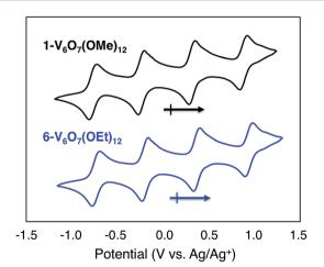
Fig. 2 Cyclic voltammograms of 1 mM solutions of complexes 1- $V_6O_7(OMe)_{12}$  (black) and  $6-V_6O_7(OEt)_{12}$  (blue) with 100 mM [NBu<sub>4</sub>] [PF<sub>6</sub>] in MeCN and a scan rate of 200 mV s<sup>-1</sup>.
