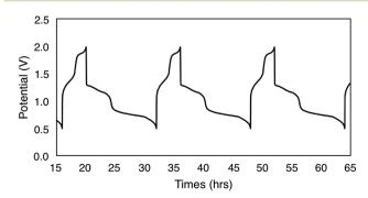
Fig. 3 Potential curves of complex  $1-V_6O_7(OMe)_{12}$  for cycles 2-4.
