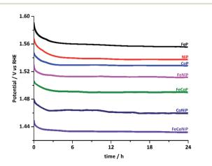
Fig. 4 Chronopotentiometric curves for TMP pre-catalysts recorded at a constant current density of 10 mA cm<sup>-2</sup>
