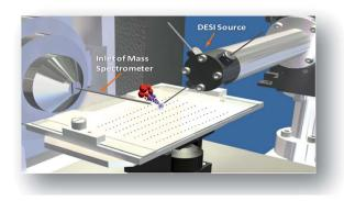
Fig. 2 Reaction (in secondary droplets) and MS product analysis of reaction mixtures presented in microtiter plate format. Automated acquisition of DESI mass spectra occurs at a rate of 1 reaction mixture per s.
