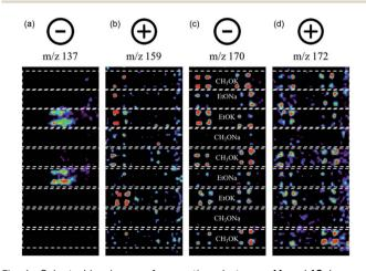
Fig. 4 Selected ion images for reactions between 11 and 12. Images. (a) Negative ion mode m/z 137, 11; (b) positive ion mode m/z 159, 12; (c) negative ion mode m/z 170, 13; (d) positive ion mode m/z 172, 13.
