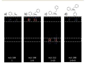
Fig. 3 Selected ion images for reactions between amines and alkyl bromides. Images are (a) m/z 108, benzylamine; (b) m/z 198, alkylation product for reaction of 1 and 9; (c) m/z 212, alkylation product for reaction of 1 and 10; (d) m/z 288, double alkylation product for reaction of 2 and 9.
