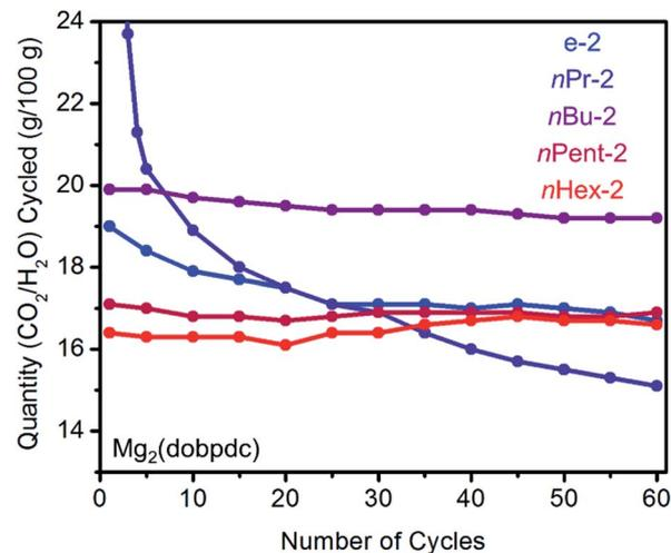
Fig. 5 Cycling stability of 1°,2°-alkylethylenediamine-appended variants of Mg<sub>2</sub>(dobpdc) in a simulated temperature swing adsorption process. Adsorption conditions: humid 15% CO<sub>2</sub> in N<sub>2</sub>, 40 °C, 5 min; desorption conditions: humid CO<sub>2</sub>, 140 °C, 5 min. Over 60 cycles, the diamine loadings decreased by 13%, 23%, 11%, 3%, and 1% for e-2, *n*Pr-2, *n*Bu-2, *n*Pent-2, and *n*Hex-2, respectively.
