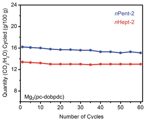
Fig. 14 Cycling stability of 1°,2°-alkylethylenediamine-appended variants of Mg<sub>2</sub>(pc-dobpdc) in a simulated CCS process. Adsorption conditions: humid 15% CO<sub>2</sub> in N<sub>2</sub>, 40 °C, 5 min; desorption conditions: humid CO<sub>2</sub>, 140 °C, 5 min. Over 60 cycles, the diamine loadings decreased by 5% for *n*Pent-2 and <1% for *n*Hept-2.
