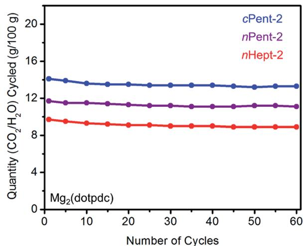
Fig. 10 Cycling stability of 1°,2°-alkylethylenediamine-appended variants of Mg<sub>2</sub>(dotpdc) in a simulated temperature swing adsorption process. Adsorption conditions: humid 15% CO<sub>2</sub> in N<sub>2</sub>, 40 °C, 5 min; desorption conditions: humid CO<sub>2</sub>, 140 °C, 5 min. Over 60 cycles, the diamine loadings decreased by 10%, 3%, and 3% for cPent-2, *n*Pent-2, and *n*Hept-2, respectively.
