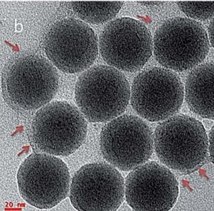
Fig. 3 TEM micrographs of UCN@SiO $_2$ -GO nanocomposite, region (a) at low magnification (b) at high magnification.
