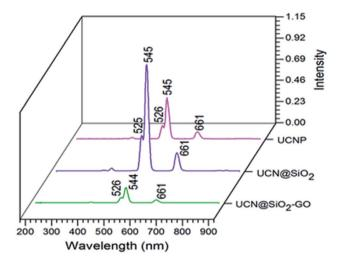
Fig. 7 Fluorescence spectra of UCNPs, UCN@SiO $_2$  NPs and UCN@SiO $_2$ –GO nanocomposite.
