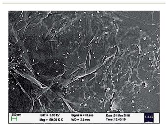
Fig. 4 Representative FESEM micrograph of UCN@SiO2-GO nanocomposite.
