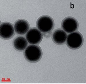
Fig. 2 TEM micrographs of (a) core shell UCN@SiO $_{\rm 2}$  NPs (b) at different region.
