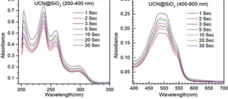
Time dependent release of DOX studied through UV-Visible absorption spectra for UCN@SiO2 NPs.
