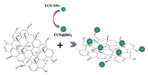
Scheme 1 Schematic showing the concept of making UCN@SiO2-GO conjugated nanocomposite. UCN@SiO2 NPs are conjugated with GO.
