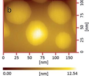
Fig. 1 (a) TEM micrograph and (b) AFM topographic image of UCNPs.
