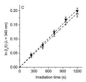
Fig. 5 First-order plots for the photooxidation of Trp (20 μM) photosensitized by (A) TCP (■) and TCP in presence of β-carotene (□), (B) TCP-C<sub>60</sub> (▲) and TCP-C<sub>60</sub> in presence of β-carotene (△) and (C) TCP-C<sub>60</sub><sup>4+</sup> (▼) and TCP-C<sub>60</sub><sup>4+</sup> in presence of β-carotene (∇) in DMF;  $\lambda_{irr} = 562$  nm.
