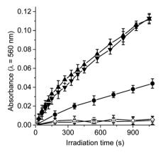
Fig. 3 Time course of NBT reduction as an increase in the absorption at  $\lambda=560$  nm in DMF/10% water. Samples contain NBT (0.2 mM), NADH (0.5 mM) and TCP-C<sub>60</sub> ( $\blacktriangle$ ) (1.2  $\mu$ M) or TCP-C<sub>60</sub>  $^{4+}$  ( $\blacktriangledown$ ) (1.2  $\mu$ M) in DMF/10% water irradiated with light at  $\lambda_{irr}=428$  nm. Controls: NBT and NADH ( $\spadesuit$ ), TCP-C<sub>60</sub> and NTB ( $\triangle$ ); TCP-C<sub>60</sub>  $^{4+}$  and NBT ( $\triangledown$ ).
