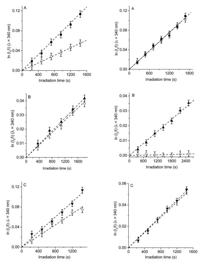
Fig. 6 First-order plots for the photooxidation of Trp (20  $\mu M$ ) in photosensitized by (A) TCP (■) and TCP in presence of sodium azide (□), (B) TCP-C<sub>60</sub> ( $\blacktriangle$ ) and TCP-C<sub>60</sub> in presence of sodium azide ( $\triangle$ ) and (C) TCP-C<sub>60</sub><sup>4+</sup> ( $\blacktriangledown$ ) and TCP-C<sub>60</sub><sup>4+</sup> in presence of sodium azide ( $\nabla$ ) in DMF/2.5% water;  $\lambda_{irr} = 562$  nm.
