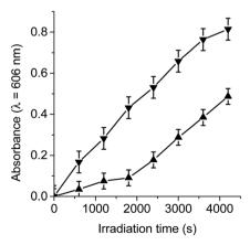
Fig. 2 Time course of MV<sup>2+</sup> (0.8 mM) reduction as an increase in the absorption at  $\lambda=606$  nm sensitized by TCP-C<sub>60</sub> (  $\blacktriangle$ ) (3.0  $\mu$ M) and TCP-C<sub>60</sub>  $^{4+}$  (  $\blacktriangledown$ ) (3.0  $\mu$ M) containing TMN (0.4 mM) after 10 min irradiation periods with light at  $\lambda_{irr}=433$  nm under an argon atmosphere in DMF/5% water.
