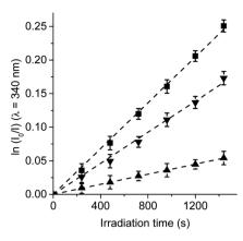
Fig. 4 First-order plots for the photooxidation of Trp (20  $\mu$ M) photosensitized by TCP ( $\blacksquare$ ), TCP-C<sub>60</sub> ( $\blacktriangle$ ) and TCP-C<sub>60</sub><sup>4+</sup> ( $\blacktriangledown$ ) in DMF;  $\lambda_{irr}$  = 428 nm.
