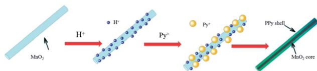
Scheme 2 Schematic illustration of the formation mechanism of the MnO<sub>2</sub>/PPy nanocomposites in acid condition.
