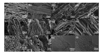
**Fig. 1** SEM images of (a and b) the printing paper, (c and d) precarbonized materials, (e and f) WPPC-2, (g and h) WPPC-3, and (i and j) WPPC-4 (g); TEM images of (k and l) WPPC-2.
