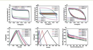
Fig. 5 Capacitive performance of the WPPCs in the KOH electrolyte: (a) CV curves of the WPPCs at 30 mV  $s^{-1}$ , (b) CV curves of the WPPC-2 at 10-500 mV s<sup>-1</sup>, (c) CV curves of the WPPCs at 500 mV s<sup>-1</sup>, (d) GCD curves of WPPCs at 0.3 A  $g^{-1}$ , (e) GCD curves of the WPPC-2 at 1-20 A g<sup>-1</sup>, (f) specific capacitances of WPPCs at different discharge current densities.
