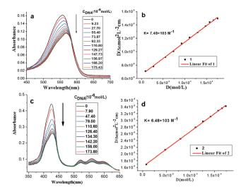
Fig. 1 UV-vis absorption spectra of compound 1 (a) and compound 2 (c) with the titration of ct-DNA; maximal absorption intensity of compound 1 (b) and 2 (d) with the titration to ct-DNA. The concentration of compound 1 and 2 is 4  $\mu$ mol L<sup>-1</sup>. Buffer solution (pH = 7.4,  $0.05 \text{ mol L}^{-1} \text{ Tris-HCl}, 0.1 \text{ mol L}^{-1} \text{ NaCl}).$
