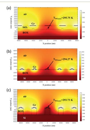
Fig. 11 Thermal field distributions of conventional structure with 1 μm-thick SiO<sub>2</sub> top cladding (a), graphene contact-heating structure without air trench (b) and with air trench (c).
