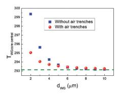
Fig. 12 Dependence of temperature at central waveguide core  $(T_{\text{WGcore central}})$  on waveguide pitch  $(d_{\text{WG}})$  with and without air trench. Dashed green line indicates the ambient temperature.
