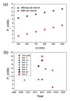
Fig. 8 (a)  $P_{\pi}$  as function of d with and without air trench. (b) Summarization of  $P_{\pi}$  reported in references.
