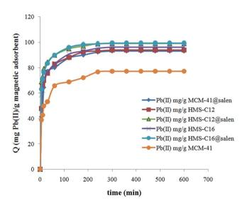
Fig. 10 Influence of contact time on  $Pb(\shortparallel)$  adsorption onto synthesized silicas.
