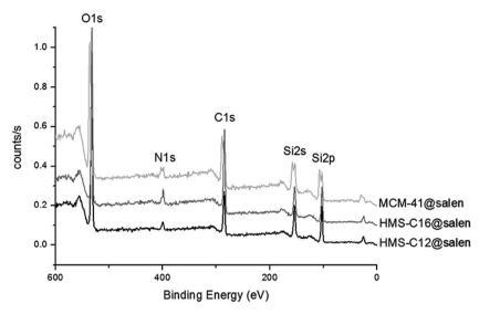
Fig. 3 XPS spectra of MCM-41@salen, HMS-C12@salen, HMS-C16@salen (the spectra were normalized and shifted on the y axis).
