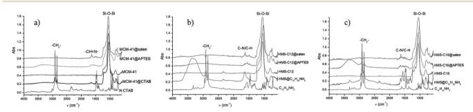
Fig. 2 FTIR spectra of (a) CTAB, MCM-41@CTAB, MCM-41, MCM-41@APTES, MCM-41@salen; (b) C<sub>12</sub>H<sub>25</sub>NH<sub>2</sub>, HMS@C<sub>12</sub>H<sub>25</sub>NH<sub>2</sub>, HMS-C12, HMS-C12@APTES, HMS-C12@salen; (c)  $C_{16}H_{33}NH_2$ , HMS@ $C_{16}H_{33}NH_2$ , HMS-C16, HMS-C16@APTES, HMS-C16@salen.
