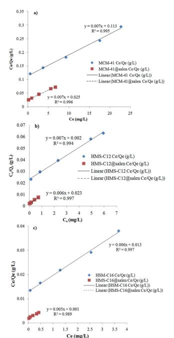
Fig. 11 Langmuir linearized isotherms for Pb(ii) sorption onto (a) MCM-41, MCM-41@salen; (b) HMS-C12, HMS-C12@salen, (c) HMS-C16, HMS-C16@salen.
