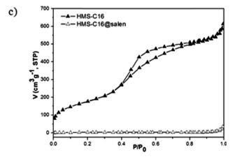
Fig. 8 Nitrogen adsorption-desorption isotherms of: (a) MCM-41, MCM-41@salen, (b) HMS-C12, HMS-C12@salen, and (c) HMS-C16, HMS-C16@salen.
