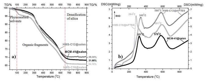
Fig. 5 (a) TG curves and (b) DSC curves of the functionalized mesoporous silicas: MCM-41@salen, HMS-C12@salen and HMS-C16@salen.
