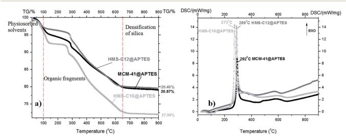
Fig. 4 (a) TG curves and (b) DSC curves of the silanized mesoporous silicas: MCM-41@APTES, HMS-C12@APTES and HMS-C16@APTES.
