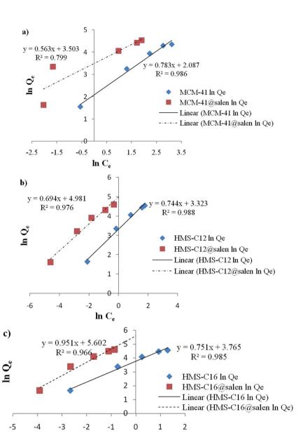
Fig. 12 Freundlich linearized isotherms for Pb(II) sorption onto (a) MCM-41, MCM-41@salen; (b) HMS-C12, HMS-C12@salen, (c) HMS-C16, HMS-C1 C16@salen.
