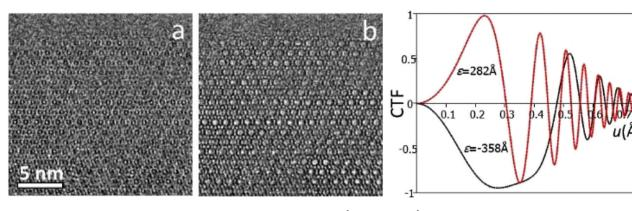
Fig. 2 HRTEM images of ITQ-39 taken along the [100] axis at defocus 282 Å (a) and -358 Å (b). Image (b) was taken close to the Scherzer defocus, therefore atomic columns are shown as black dots. The contrast transfer functions of (a) and (b) are shown in (c).
