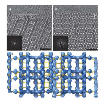
Fig. 9 Structure projection images reconstructed from 20 HRTEM images along (a) [010] and (b) [100] of ITQ-39. 10-ring channels are observed in (b), and the channel stacking is traced by a line in (b). The domains used for structure factor determination are outlined by the rectangles. (c) The 3D electrostatic potential map reconstructed from the structure factor amplitudes and phases extracted from the marked nano domains in (a) and (b).18
