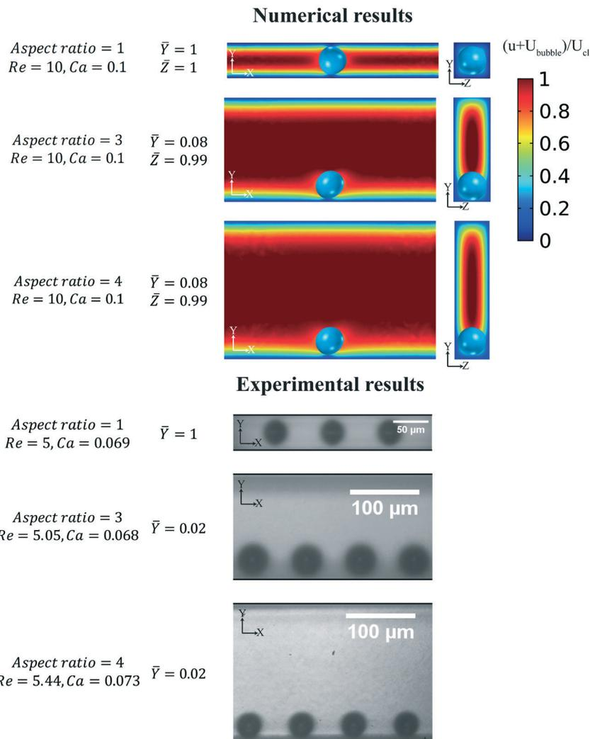
**Fig. 10** Effect of the channel geometry on the lateral position of the bubble while the  $Re$  and  $Ca$  are constant. Experimental and numerical results show that in the wider channels, the bubble equilibrium position is close to the smaller edge while in the channel with an aspect ratio of one the bubble equilibrium position is in the center.
