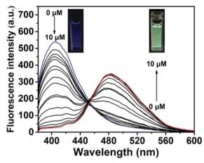
Fig. 2 Changes in fluorescence emission of ABAH-LW (3  $\mu$ M) with increasing addition of ONOO $^-$  (from 0 to 10  $\mu$ M) in PBS buffer (pH 8.2, containing 8% DMSO, 1 mM CTAB) after 1 min.  $\lambda_{ex}$  = 370 nm. Slit widths: ex = 5 nm. em = 6 nm.
