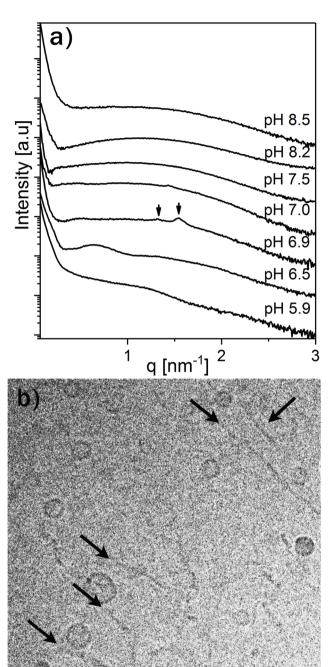
Fig. 6 (a) SAXS patterns at increasing pH for OA emulsions loaded with 30 wt% LL-37 and stabilized by F127. Identifiable Bragg reflections from a potential micellar cubic Fd3m phase at pH 6.9 are marked with arrows. (b) Representative cryo-TEM image of the corresponding dispersion at pH 8.5. Thin thread-like cylindrical micelles and/or bilayer fragments (marked with arrows) coexisting with small vesicles were observed.
