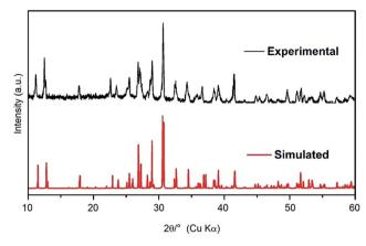
Fig. 1 Experimental and simulated powder X-ray diffraction patterns of the Na<sub>2</sub>Tb<sub>1.08</sub>Ca<sub>2.92</sub>Si<sub>6</sub>O<sub>18</sub>H<sub>0.8</sub> compound. The simulated pattern is based on the structure refined by our single-crystal X-ray diffraction analysis.
