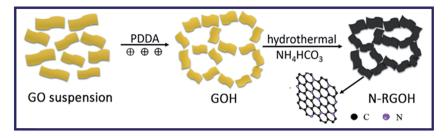
Fig. 10 Schematic diagram of the formation mechanism for the nitrogen doped graphene hydrogel.<sup>85</sup>
