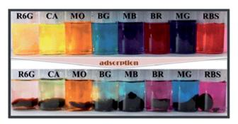
Fig. 7 Photographs of different dye solutions before and after adsorption by the GO/SA/PAM composite hydrogels.<sup>65</sup>
