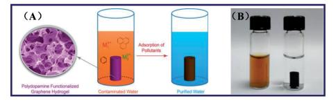
Fig. 4 (A) Microstructure and adsorption process of the graphene hydrogel, and (B) photograph of GO dispersion mixed with dopamine (left) and the monolithic material of PDA-GH (right).<sup>56</sup>
