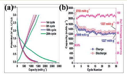
Fig. 16 (a) Galvanostatic plots for the charge/discharge cycle performance and (b) coulombic efficiency of the B-G electrode at a low current rate of 50 mA g<sup>-1</sup> between 3.0 and 0.01 V versus Li<sup>+</sup>/Li. Reproduced with permission.<sup>156</sup> © 2011 American Chemical Society.
