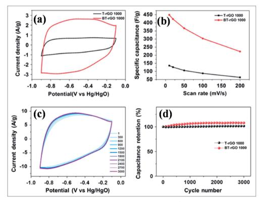
Fig. 15 (a) Cyclic voltammetry (CV) curves for T-rGO and BT-rGO at a scan rate of 10 mV s<sup>-1</sup>, (b) specific capacitances as a function of scan rate, (c) CV curves for 3000 cycles at a scan rate of 50 mV s<sup>-1</sup>, and (d) retained capacitance as a function of cycle number of T-rGO and BT-rGO electrodes. Reproduced with permission.  $^{172}$  © 2015 Nature Publishing Group.
