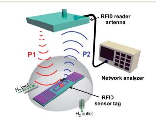
Fig. 9 Schematic diagram of the UHF-RFID-based wireless sensor system showing transmission between the RFID sensor tag and RFID reader antenna connected to a network analyzer. [Reprinted with permission from ref. 187 Copyright © American Chemical Society.]
