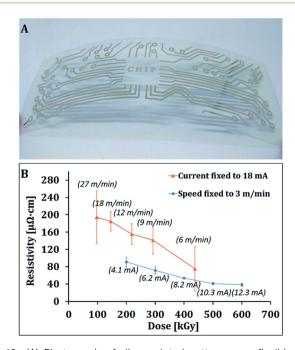
Fig. 18 (A) Photograph of silver printed pattern on a flexible PEN substrate after electron beam (ebeam) sintering process. (B) Change of resistivity as a function of energy dose. Effects of conveyor speed at fixed current of 18 mA and current at fixed speed of 3 m  $min^{-1}$  on the resistance of printed silver patterns. The voltage was fixed at 110 kV. [Reprinted with permission from ref. 232 Copyright © The Royal Society of Chemistry.]
