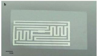
Fig. 25 (a) Photograph of inkjet printed silver patterns on PET substrate showing the metallic luster. (b) Inkjet printed silver ink based RFID antenna. [Reprinted with permission from ref. 120 Copyright © Elsevier.]
