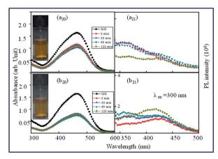
Fig. 22 Photocatalytic and photoluminescence spectra of silicacoated anatase- and rutile-TiO<sub>2</sub> nanoparticles. UV-Vis spectra of the photodegradation of methyl orange dye by anatase\_silica (a20) and rutile\_silica ( $b_{20}$ ), respectively, at various time intervals. ( $a_{21}$ ) and ( $b_{21}$ ) show the PL characteristics of anatase\_silica and rutile\_silica, respectively.<sup>23</sup> Reprinted with permission from ref. 23. Copyright 2016. Elsevier.
