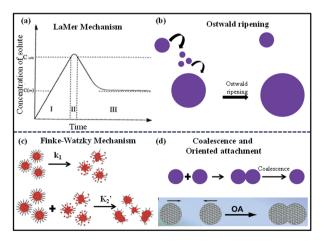
Scheme 3 Different possible growth mechanisms for the synthesis of nanostructured  $TiO_2$  materials. (a) is reprinted with permission from ref. 325. Copyright 2014. American Chemical Society. (c) is reprinted with permission from ref. 326. Copyright 2015. The Royal Society of Chemistry.
