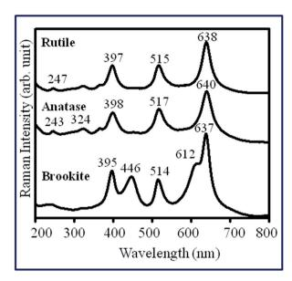
Fig. 18 Raman spectra of brookite-, anatase- and rutile- $TiO_2$  nanoparticles.<sup>275</sup> Reprinted with permission from ref. 275. Copyright 2015. VBRI Press.
