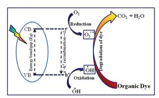
Fig. 3 Photocatalysis mechanism in multiphase TiO<sub>2</sub> nanostructures.
