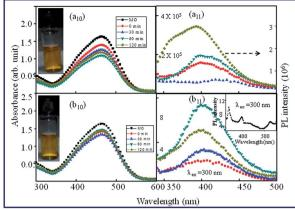
Fig. 21 Photocatalytic and photoluminescence spectra of anataseand rutile-TiO<sub>2</sub> nanoparticles. UV-Vis spectra of the photodegradation of methyl orange dye by anatase (a20) and rutile (b20), respectively, at various time intervals. (a21), and (b21) show the PL characteristics of anatase and rutile, respectively at  $\lambda_{ex} = 300$  nm.<sup>23</sup> Reprinted with permission from ref. 23. Copyright 2016. Elsevier.
