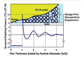
Fig. 3 Schematic shows nanoparticle wedge film confined by solid surface and oil-nanofluid interface and relationship between disjoining pressure and film thickness. (Reprinted with permission from (ref. 32). Copyright (2014) American Chemical Society.)
