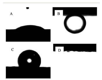
Fig. 1 Wetting conditions for rock surface in different phases ((A) air/water, (B) water/n-heptane) and a carbonate rock aged in the oil ((C) air/water, (D) water/n-heptane). (Reprinted with permission from (ref. 11). Copyright (2012) American Chemical Society.)
