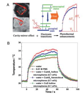
Fig. 3 (A) Schematic demonstration of photothermal conversion enhancement and temperature elevation based on the cavity-mirror effect and interband transitions. (B) Temperature elevation of water, PBS and different superstructures under laser irradiation.<sup>76</sup> Reprinted with permission from ref. 76. Copyright 2013 American Chemical Society.
