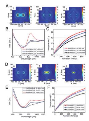
Fig. 11 Electric field distribution of Au nanorod@ $Cu_7S_4$  hybrid with different shell thickness ((A) a, 8.8 nm; b, 12.1 nm; c, 15.1 nm) and size ((D) a, 90.1 nm; b, 157.4 nm; c, 256.2 nm) in FDTD simulation. (B, E) The LSPRs absorption spectra and (C, F) photothermal profiles for Au nanorod@ $Cu_7S_4$  hybrid with different shell thickness and size.<sup>49</sup> Reprinted with permission from ref. 49. Copyright 2016 American Chemical Society.
