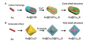
Fig. 1 Scheme of synthesizing the  $Au-Cu_{2-x}S$  hybrid based on the template method. (4),63 (A) Reprinted with permission from ref. 63. Copyright 2016 Wiley-VCH Verlag & Co. KGaA. (B) Reprinted with permission from ref. 49. Copyright 2016 American Chemical Society.
