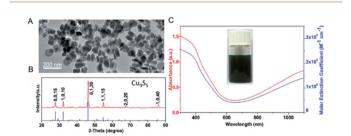
Fig. 8 TEM image (A), and XRD (B), absorption (C, red) and molar extinction coefficient (C, blue) of the prepared Cu<sub>9</sub>S<sub>5</sub> NPs.<sup>19</sup> Reprinted with permission from ref. 19. Copyright 2011 American Chemical Society.
