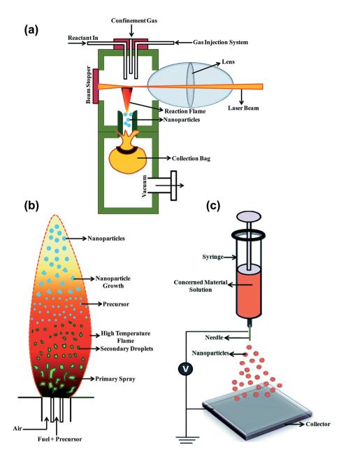
Fig. 10 Schematic diagrams of (a) laser pyrolysis, (b) flame spray pyrolysis and (c) an electrospraying technique for the synthesis of nanoparticles.<sup>80</sup>
