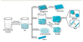
Fig. 9 Schematic illustration of sol-gel processes.<sup>75</sup>
