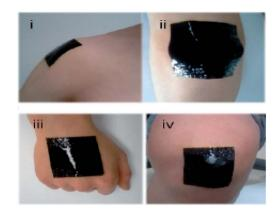
Fig. 27 Photographic images of the HSNG at various locations on the human body (i) shoulder (ii) elbow (iii) dorsal side of hand (iv) knee showing the good compatibility of the device.<sup>251</sup>
