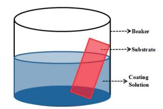
Fig. 14 Schematic of dip coating technique.
