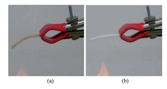
Fig. 17 Thermal stability of (a) paper-based nanogenerator and (b) polymer-based nanogenerator.<sup>243</sup>
