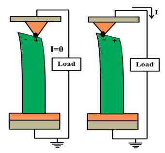
Fig. 3 Operating principle of PENG and formation of a Schottky contact with the application of a perpendicular force.
