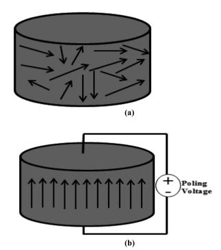
Fig. 16 (a) Before poling. (b) After poling
