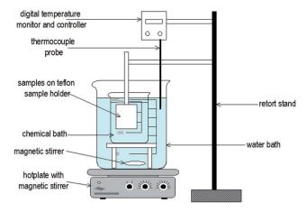
Fig. 8 Experimental setup used for chemical bath deposition. 68
