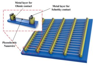
Fig. 4 Basic structure of LING
