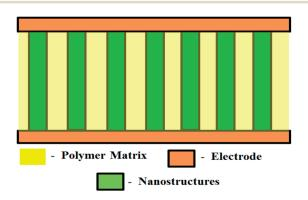
Fig. 5 Schematic diagram of NEG.
