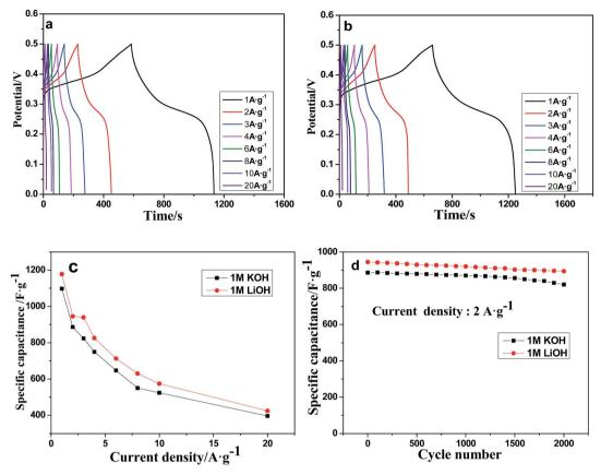
Fig. 6 The charge–discharge curves of the Mn-LMOF electrode at different current densities (a) 1 M KOH (b) 1 M LiOH. (c) The curves of specific capacitance *versus* current density in 1 M KOH and 1 M LiOH. (d) Cycle life diagrams of the Mn-LMOF electrode at 2 A  $g^{-1}$  in 1 M KOH and 1 M LiOH.
