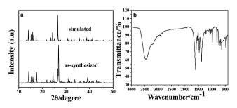
Fig. 1 (a) XRD pattern of as-synthesized Mn-LMOF and the simulated pattern based on the crystal data of Mn-LMOF (b) FT-IR spectrum of the Mn-LMOF.
