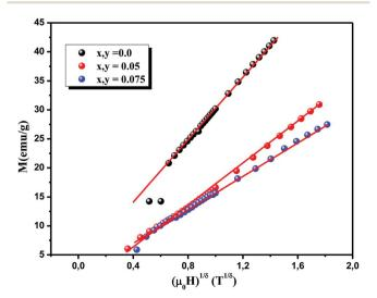
Fig. 11 The linearity of the  $M(T=T_{\rm C})$  versus  $\mu_0 H^{\beta/(\beta+\gamma)} = \mu_0 H^{1/\delta}$  curves validates the value of  $\delta$  calculated using the Widom relationship with the experimental data.
