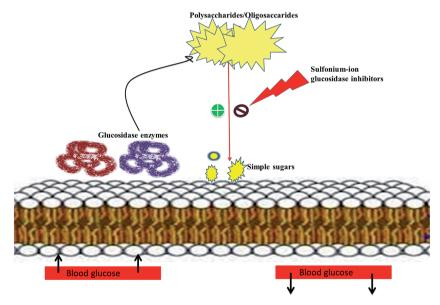
Fig. 2 Pictorial depiction showing mechanism of sulfonium-ion as α-glucosidase inhibitors.
