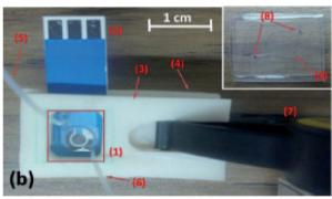
Fig. 14 (a) Schematic illustration of the setup of a device stack, (b) optical photograph of an as-constructed microfluidic NEGS device: (1) PDMS chamber (inset (b): enlarged view), (2) Ni/CS/rGO/SPE, (3) top and (4) bottom pieces of plastic device holder, (5) outlet tube, (6) inlet tube joined with sample injector, (7) microbar clamp/spreader, (8) holes for joining the outlet and inlet tubes, (9) circular chamber (reproduced with permission from Elsevier; Yang et al. 2013).
