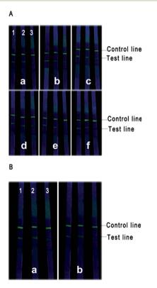
Fig. 6 The stability of strips. 1, 2 and 3 represented the different concentrations of *E. coli* O157:H7, namely  $10^6$  CFU mL $^{-1}$ ,  $10^5$  CFU mL $^{-1}$  and  $10^4$  CFU mL $^{-1}$ , respectively (A) The results of strips for the detection of *E. coli* O157:H7 after storing for 0 d (a), 7 d (b), 14 d (c), 21 d (d), 28 d (e) and 35 d (f) (B) the diagrams of the used strips after storing for 0 d (a) and 20 d (b).
