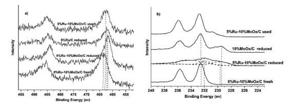
Fig. 2 XPS spectra of Ru-MoO $_x$ /C catalysts: (a) Ru 3p and (b) Mo 3d. 5% Ru-10% MoO $_x$ /C fresh: the catalyst had not been reduced by H $_2$ ; 5% Ru-10% MoO $_x$ /C and 5% Ru/C reduced: the catalysts were reduced by H $_2$  under 350 °C; 5% Ru-10% MoO $_x$ /C used: the catalyst was reduced by H $_2$  under 350 °C and then used at the reaction condition.
