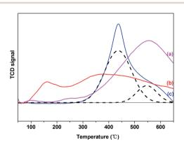
Fig. 1  $H_2$ -TPR profiles of (a) 5% Ru/C, (b) 5% Ru-10% MoO<sub>x</sub>/C and (c) 10% MoO<sub>x</sub>/C catalysts.
