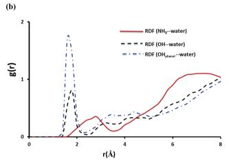
Fig. 13 The RDF of hydrogen bonding interactions for NP $-\beta$ CD-18C6 complex plotted as a function of separation distance r (in Å) between donor and acceptor. (a) Represents interaction of NP with the two hosts. (b) Represents interaction of NP with water.
