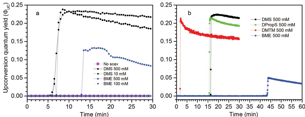
Fig. 3 The measured  $\Phi_{UC}$  in filled screw-cap vials during continuous irradiation at 532 nm. (a) High concentration TTA-UC system ( $[PdOEP] = 16 \mu M$  and  $[DPA] = 500 \mu M$ ) and (b) lower concentration system ( $[PdOEP] = 5 \mu M$  and  $[DPA] = 100 \mu M$ ).
