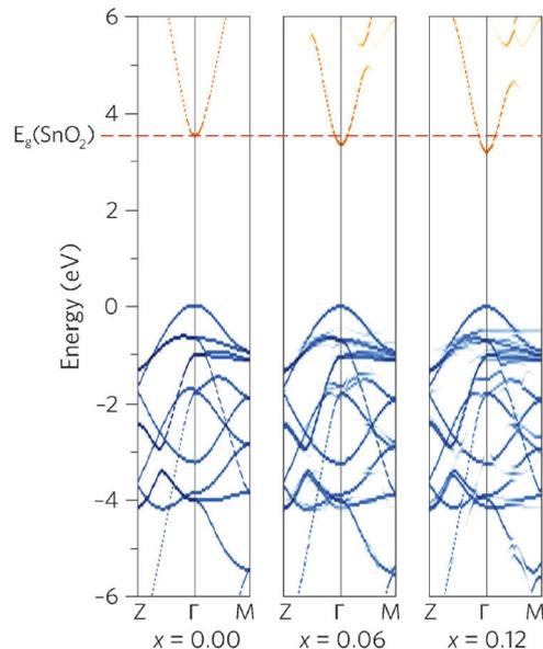
Fig. 3 The calculated effective band structure for  $\text{Sn}_{1-x}\text{Pb}_x\text{O}_2$  where  $x = 0.00, 0.06,$  and  $0.12$ . The conduction bands are coloured orange whereas the valence bands are shown in blue, with the VBM is set to 0 eV in each case.
