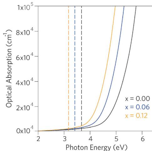
Fig. 5 Calculated optical absorption spectra for  $\text{Sn}_{1-x}\text{Pb}_x\text{O}_2$  where  $x = 0.00, 0.06,$  and  $0.12$ . Full lines indicate optical absorption and dashed lines indicate fundamental band gap.
