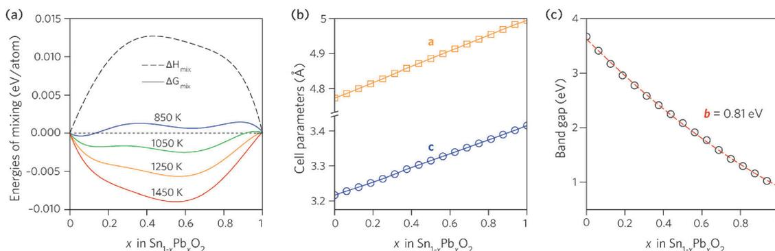
**Fig. 2** Trends across the full composition space of  $\text{Sn}_{1-x}\text{Pb}_x\text{O}_2$  for: (a) the enthalpy and free energy of mixing, (b) the unit cell lattice parameters, and (c) the direct fundamental band gaps ( $E_g^{\text{dir}}$ ).
