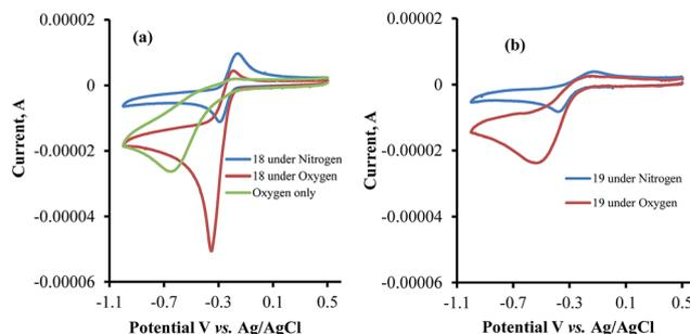
Fig. 5 (a) Cyclic voltammograms of  $\beta$ -lapachone 18 in Tris buffer under nitrogen and oxygen atmospheres and that of the oxygen saturated solution without 18. (b) Cyclic voltammograms of dehydro- $\alpha$ -lapachone 19 in Tris buffer under nitrogen and oxygen atmospheres.
