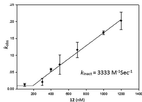
Fig. 3 Plot of the inactivation rate constants ( $k_{\text{obs}}$ ) vs. the concentration of **12** (nM), for obtaining the maximal rate of enzyme inactivation ( $k_{\text{inact}}$ ). Each value represents the mean  $\pm$  SE of two independent experiments.
