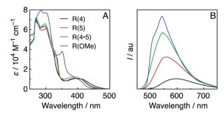
Fig. 1 UV-vis (A) and emission (B) spectra of the Re-rings in DMF under Ar. The emission spectra were corrected to the absorbed photons at  $\lambda_{ex} = 400 \text{ nm}$ .
