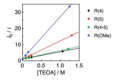
Fig. 3 Stern–Volmer plots obtained from the emission quenching of R(X) using TEOA in DMF under Ar;  $\lambda_{\rm ex}=400$  nm.
