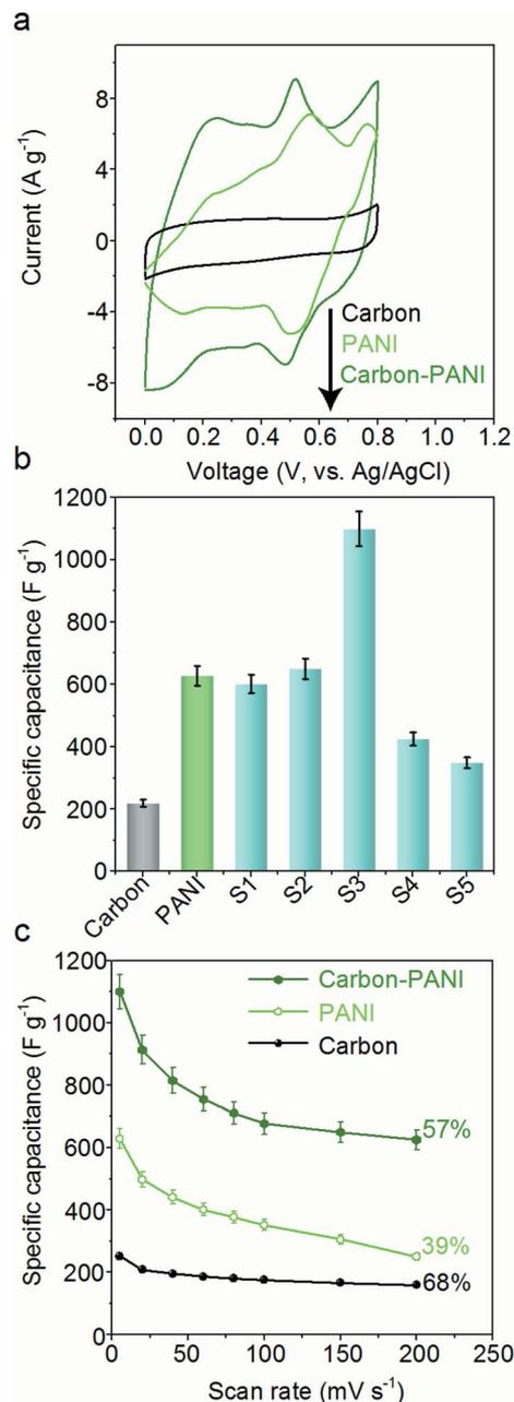
Fig. 4 Supercapacitor characterization. (a) Comparative CVs of carbon, PANI and carbon–PANI (composition S3) samples at a scan rate of 5 mV s<sup>-1</sup>. (b) Comparison of the specific capacitance performances of carbon, PANI and carbon–PANI nanocomposites (S1–S5) at various time intervals. (c) Variation of capacitance with scan rate for carbon, PANI and carbon–PANI nanocomposite (composition S3) samples.
