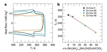
Fig. 2 DSC data (a) and phase transition temperatures (b) as a function of x in  $[\mathrm{NH_3NH_2}]_{1-x}[\mathrm{NH_3OH}]_x\mathrm{Zn}(\mathrm{HCOO})_3$ . The dotted red line acts as a guide for the eye.
