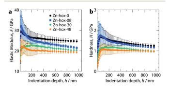
Fig. 4 Elastic moduli, E (a) and hardness, H (b) as a function of indentation depth, h along [110]. With increasing x in  $[NH_3NH_2]_{1-x}$ - $[NH_3OH]_xZn(HCOO)_3$ , the elastic modulus and hardness decrease monotonically due to reduced hydrogen bonding interactions upon substitution.
