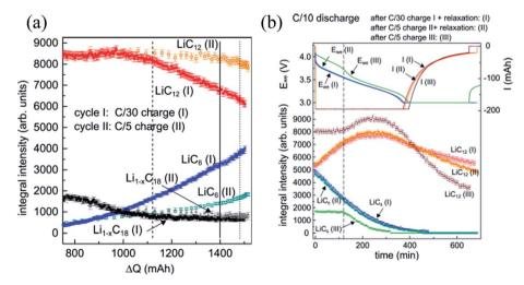
Fig. 5 (a) Integral reflection intensities of LiC<sub>6</sub>, LiC<sub>12</sub>, and Li<sub>1-x</sub>C<sub>18</sub> during C/30 (I) and C/5 (II) charging; (b) integral reflection intensity of LiC<sub>6</sub>,  $LiC_{12}$ , and  $Li_{1-x}C_{18}$  during C/10 discharging after C/30 charging + 20 h rest (I), C/5 charging + 20 h rest (II) and 5/C charging + no rest (III) (adapted from ref. 95).
