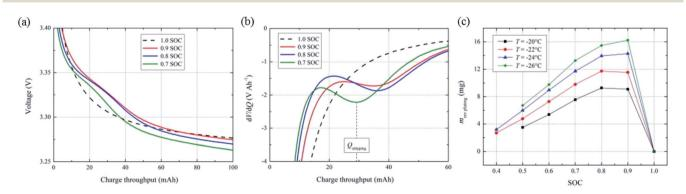
Fig. 2 (a) Discharge voltage profiles and (b) differential voltage plots (dV/dQ) of the 26650-type LiFePO<sub>4</sub>/graphite battery after 1 C charging to different SOC levels at -20 °C, and (c) reversible lithium calculated from the dV/dQ plots (adapted from ref. 10).
