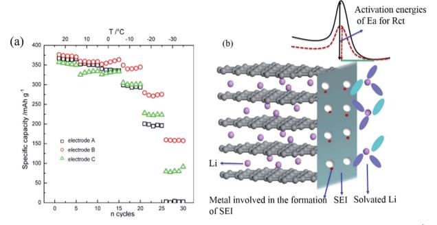
Fig. 9 (a) Reversible capacity of different graphites at C/5 from 20  $^{\circ}$ C to -30  $^{\circ}$ C: pristine oxidized graphite anode (A), coated with a 50 Å Sn layer (B) and 1% (w/o) Sn powder in oxidized graphite (C); (b) illustration of the superior performance of Sn coated graphite ((a) adapted from ref. 186).
