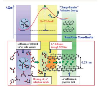
Fig. 6 Li ion intercalation process and energy barrier for charge transfer from the electrolyte to bulk graphite (adapted from ref. 116).
