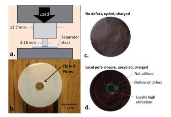
Fig. 8 (a) Schematic of a device designed to deliberately create local deformation on the separator, (b) photograph of the local-defect separator showing that the deformed part appears transparent, (c) cell with a defect-free separator in the charged state, showing uniform color, and (d) cell with a defect-containing separator in the lithiation state, showing local plating around the defect (adapted from ref. 106).
