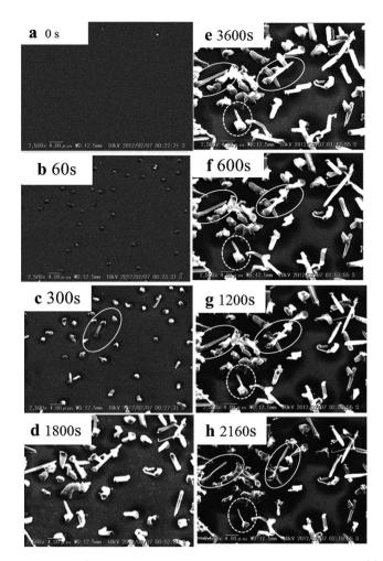
Fig. 4 In situ SEM studies of morphology during lithium plating for (a) 0 s, (b) 300 s, (c) 600 s, (d) 1800 s, and (e) 3600 s (also 0 s of stripping); stripping at 50 mA cm $^{-2}$  for (f) 600 s, (g) 1200 s, and (h) 2160 s (adapted from ref. 71).
