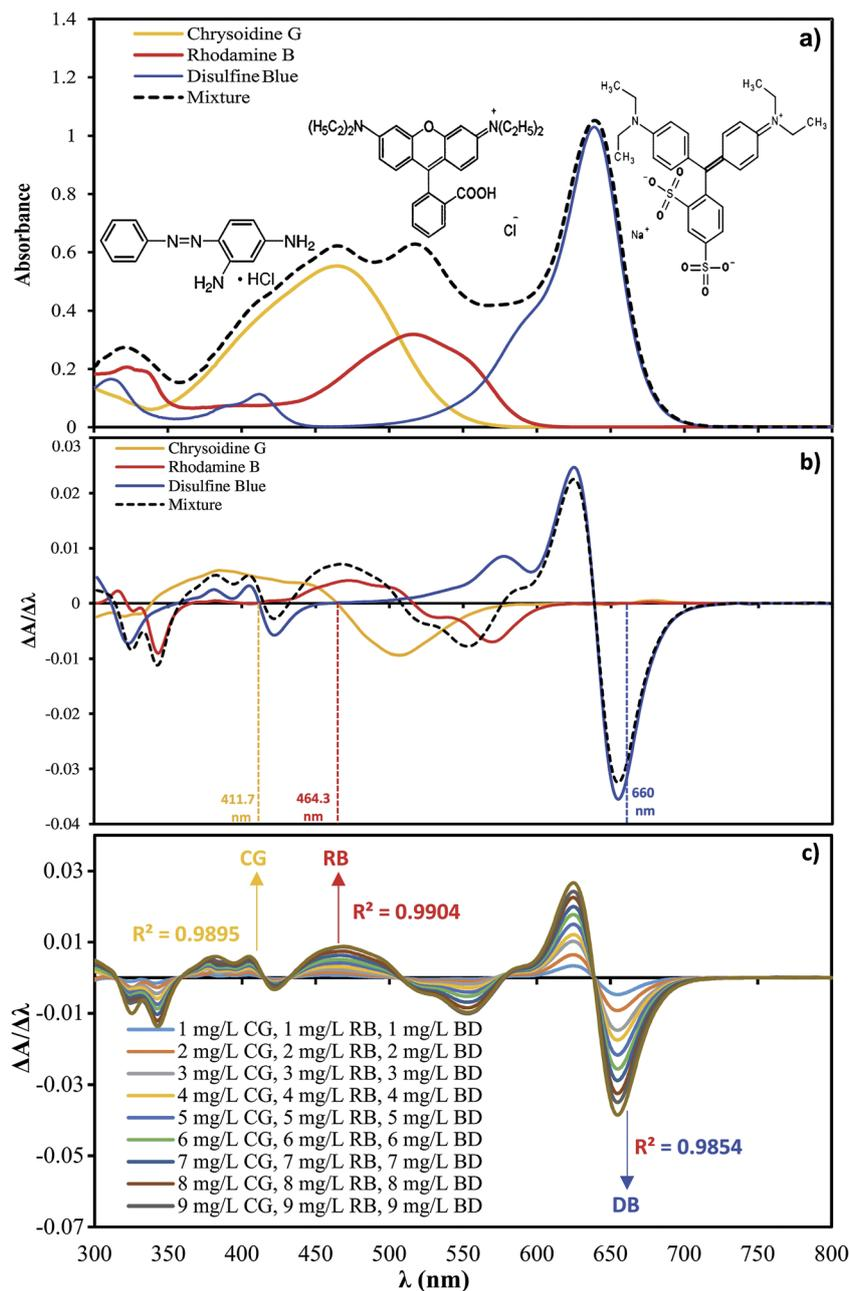
Fig. 1 (a) Zero order derivative spectra for CG, RB, DB and ternary mixture. (b) First order derivative spectra for CG, RB, DB and ternary mixture. (c) Calibration graph at 411.7 nm for CG, 464.3 for RB and 660 nm for DB.
