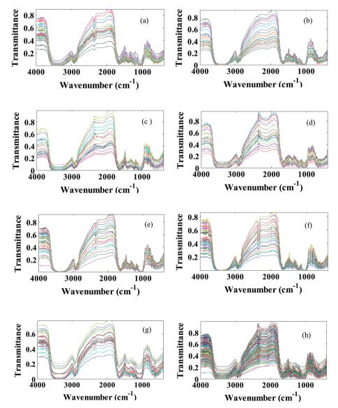
Fig. 2 Transmittance FT-IR spectra of the saffron samples used in this study: (a) standard saffron (b) Azorubine (c) Quinoline yellow (d) Allura red (e) Sudan II (f) Sunset yellow (q) Tartrazine (h) extended multiplicative scatter correction preprocessed saffron data set.
