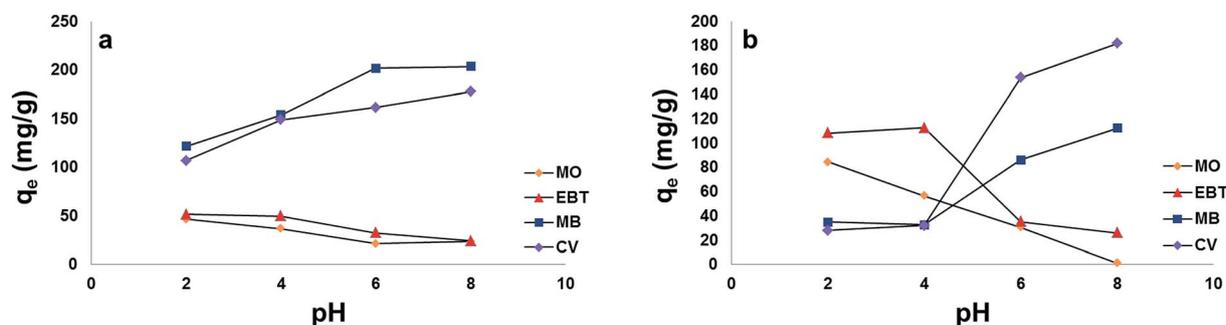
Fig. 12 Effect of pH on the adsorption capacity ( $q_e$ ) of model dyes in their mixture solutions onto; [a] MSP NPs and [b] MP NPs. Adsorbent:  $2 \text{ g L}^{-1}$ , dyes  $165 \text{ mg L}^{-1}$ , temperature:  $25^\circ \text{C}$ , time: 120 min. Magnetite/Pectin Nanoparticles: MP NPs and Magnetite/Silica/Pectin Nanoparticles: MSP NPs.
