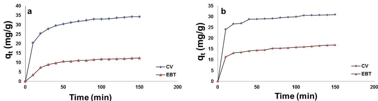
Fig. 7 Effect of contact time on the adsorption capacity ( $q_t$ ) of EBT and CV onto; [a] MSP NPs and [b] MP NPs. Adsorbent:  $2 \text{ g L}^{-1}$ , dyes  $100 \text{ mg L}^{-1}$ , temperature:  $25 \text{ }^\circ\text{C}$ , pH: natural pH of dye, time: 150 min. Magnetite/Pectin Nanoparticles: MP NPs and Magnetite/Silica/Pectin Nanoparticles: MSP NPs.
