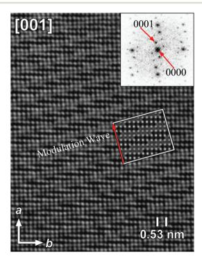
Fig. 3 [001] HRTEM image and the corresponding FT pattern of the incommensurately modulated KNd(MoO<sub>4</sub>)<sub>2</sub>. The inset represents a calculated image based on the model, for a focus value of -60 nm and a thickness of 2 nm. Reproduced with permission from ref. 23. Copyright 2006 American Chemical Society.
