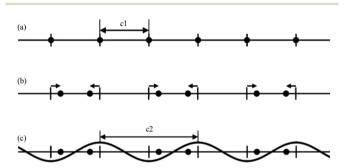
Fig. 1 A simple 1D modulated system. (a) Before modulation: all atoms (filled circles) lie equally spaced along a straight line. (b) After modulation: half the atoms shift to the left, and half to the right (arrows). (c) Modulation in (b) represented as a simple cosine function. Reproduced with permission from ref. 16. Copyright 2007 Wiley-VCH.
