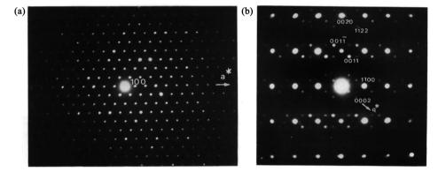
Fig. 10 Electron diffraction pattern of Ba<sub>0.85</sub>Ca<sub>2.15</sub>In<sub>6</sub>O<sub>12</sub>. (a) [001] zone axis. (b) [100] zone axis showing extra spots appearing near the main spots of the hexagonal lattice. Reproduced with permission of the International Union of Crystallography from ref. 103.
