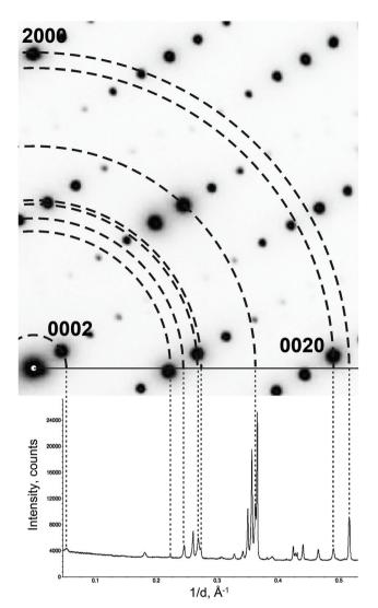
Fig. 5 Projecting an electron diffraction pattern on a powder X-ray diffraction pattern. Note that not all reflections on the powder pattern are present on the electron diffraction pattern. These reflections belong to other reciprocal lattice sections. Reproduced with permission of the International Union of Crystallography from ref. 27.
