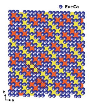
Fig. 8 Outline of cation-vacancy ordering in the  $7a \times 9b \times 1c$  commensurate approximant. WO<sub>4</sub> tetrahedra are not shown. The dimers (marked in orange) and trimers (marked in yellow) of the vacant cationic columns are marked with red rectangles. Reproduced with permission from ref. 66. Copyright 2013 American Chemical Society.
