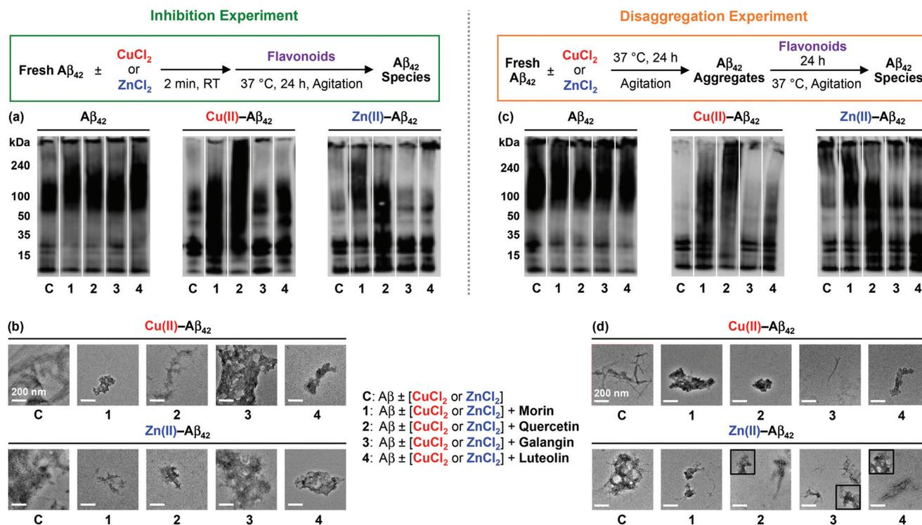
**Fig. 3** Effects of the flavonoids on metal-free and metal-induced  $A\beta_{42}$  aggregation. Top: schemes of inhibition (left) and disaggregation (right) experiments. The resultant  $A\beta_{42}$  species from the inhibition (a and b) and disaggregation (c and d) studies were visualized by gel/Western blot with an anti- $A\beta$  antibody (6E10) and TEM. The procedures and conditions are described in Fig. 2 and in the Experimental section.
