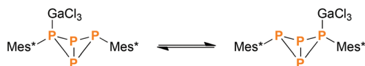
Scheme 7 In case of 5\mathbf{a}\cdot\text{GaCl}_3 , a fast intramolecular exchange of the \text{GaCl}_3 unit was observed. The Gibbs energy of activation for this process was determined to be 39.5 \text{ kJ mol}^{-1} .
