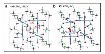
Fig. 3 Optimized geometry structures for  $4MAPbI_3 \cdot 1H_2O$  (a) and  $4MAPbI_3 \cdot 1O_2$  (b). Pb = light blue, I = violet, green = carbon, blue = nitrogen, red = oxygen, white = hydrogen.
