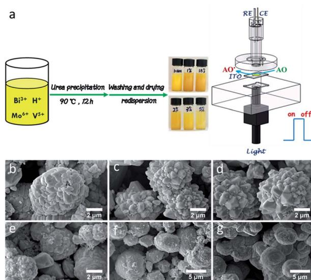
Fig. 1 (a) Schematic illustration for the preparation of  $\text{BiMo}_x\text{V}_{(1-x)}\text{O}_4$  and the PEC process for the AC assay. FESEM images of  $x =$  (b) 0, (c) 0.01, (d) 0.015, (e) 0.02, (f) 0.03 and (g) 0.05 for  $\text{BiMo}_x\text{V}_{(1-x)}\text{O}_4$ .
