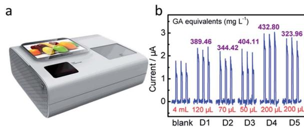
**Fig. 6** (a) Photograph of the integrated PEC platform. (b) Photocurrent responses of the  $\text{BiMo}_{0.015}\text{V}_{0.985}\text{O}_4$  modified ITO electrode in the integrated PEC platform without (blank PBS solution) and with the addition of a certain volume of juice to 4 mL of  $0.1 \text{ mol L}^{-1}$  PBS ( $\text{pH} = 7.4$ ).
