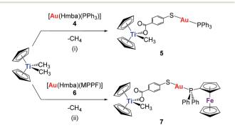
Scheme 1 Preparation of heterometallic titanocene–gold complexes  $[(\eta-C_5H_5)_2Ti(CH_3)\{OC(O)C_6H_4SAu(PR_2R')\}]$  (R = R' = Ph, 5; R = Ph, R' = ferrocene, 7). (i) THF/toluene 1.5 : 1, RT, 1 h; (ii) acetonitrile/toluene 3 : 1, RT, 1 h.
