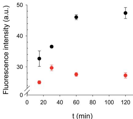
Fig. 5 Fluorescence intensity of BODIFLOXACIN when MIP microspheres were deposited onto fiber microwell arrays and incubated at different times in absence (black points,  $B_0$ ,  $n = 2$ ) and in presence of ENRO (red points, [ENRO] = 8.3  $\mu\text{M}$ ,  $n = 2$ ).
